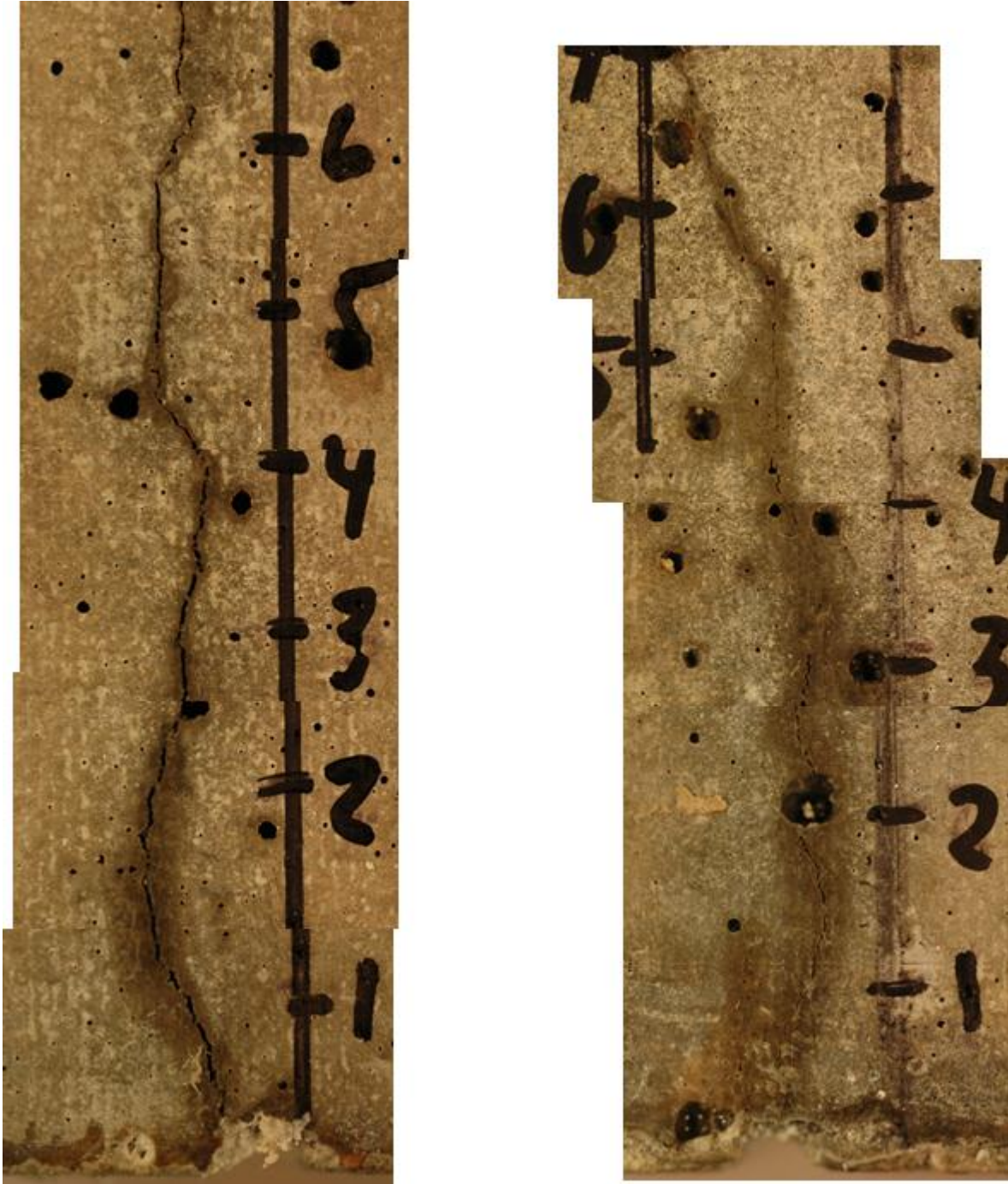
Figure 12.1: Photographs of cracks after exposure. The same specimens as in figure 7.1.
