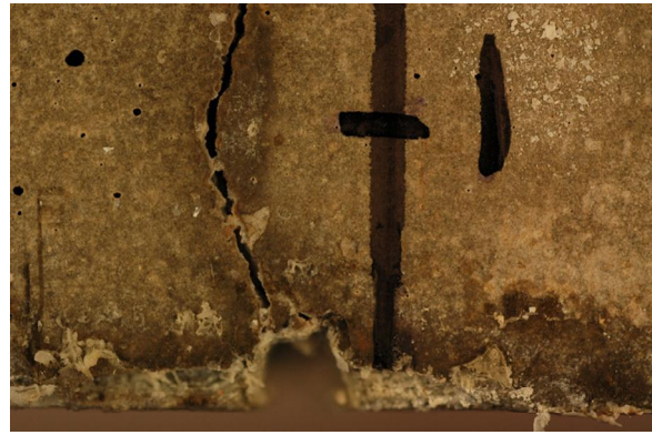
28 month exposure Specimen H55-4-2-2
