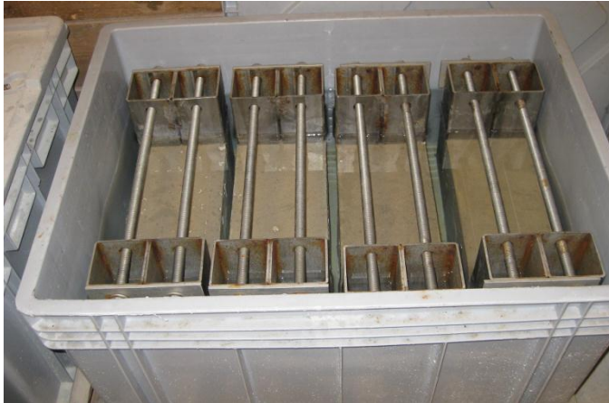
Figure 10.1: Water exposure type 1; permanently under water.
