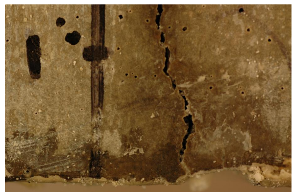
28 month exposure Specimen H55-4-1-2
