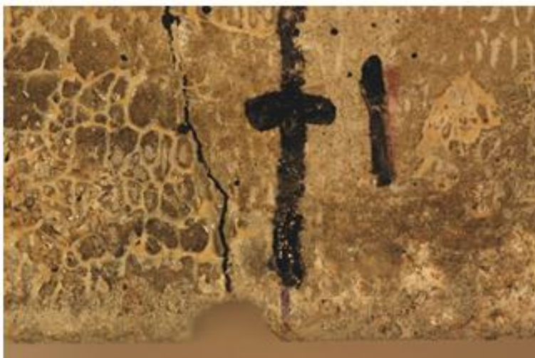
Figure 12.2: 0.2 mm crack after 28 month exposure to sea water. Concrete cover 75 mm.
