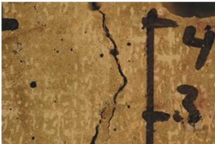
Figure A2.2: 0.4 mm crack width. 75 mm cover. Exposure to sea water.
