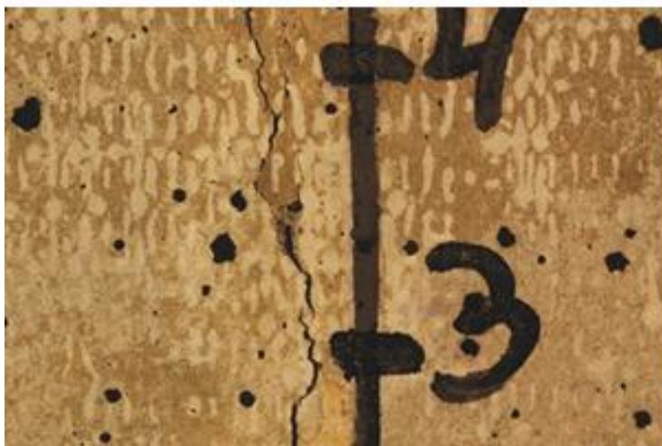
Figure A2.1: 0.2 mm crack width, 75 mm cover. Exposure to sea water.
