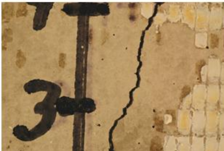
Figure A2.4: 0.4 mm crack width. 55 mm cover. Exposure to sea water.
