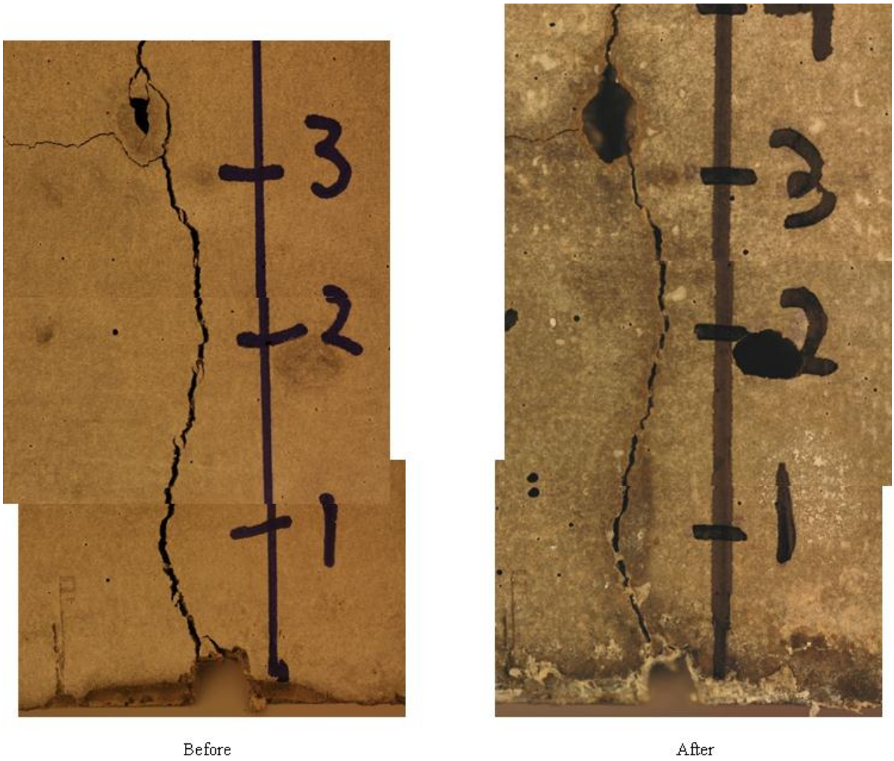
Figure A1.8: Cyclic immersion in sea water and drying. Crack width 0.4 mm. Cover 55 mm. Specimen H55-4-2-2
