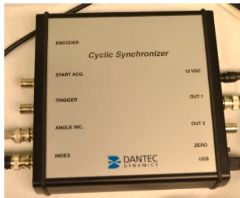
Figure 4.38. A timing box used for synchronisation in PIV measurement.
