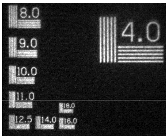
Figure 4.11. Image of a test chart to evaluate the spatial resolution of the optical setup.
