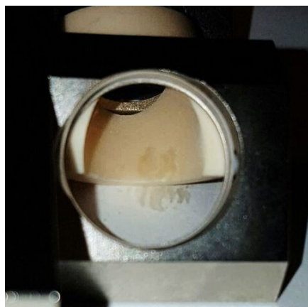
Figure 2.17. Photo of a damaged mirror in the OPO.
