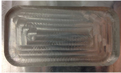
Figure 2.1 Milling task where a rectangular area of material, referred to as a pocket, is to be removed.
