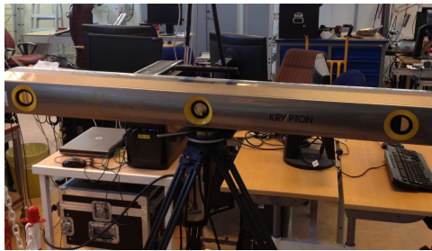
Figure 2.2 Experimental setup for milling experiments (left) at Lund University, including an optical tracking system (right) for high-accuracy measurements of robot position and orientation.
