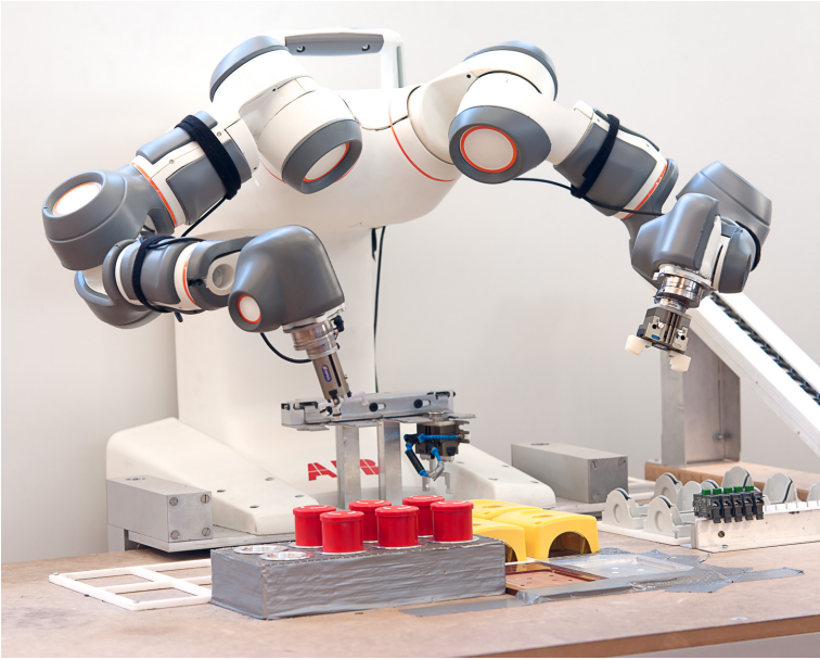
Figure 2.3 The ABB YuMi robot used in experiments in this thesis. The robot is in this photo equipped with wrist-mounted ATI Mini40 force/torque sensors.
