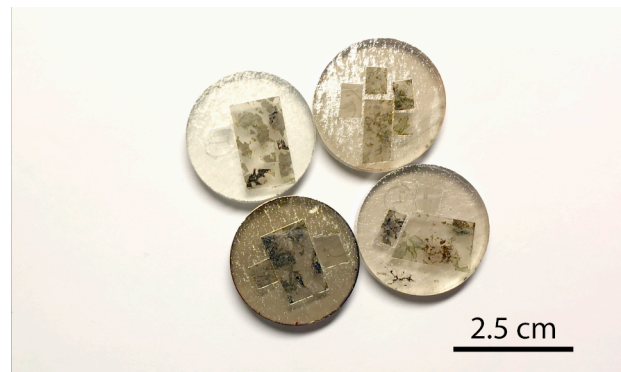
Figure 8. Thin-sections mounts for SIMS analysis.
