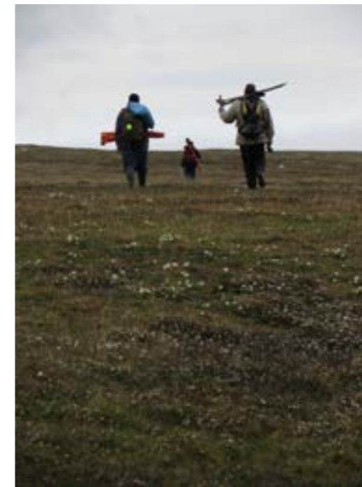
Figure 6. Field work in Adventdalen, Svalbard. The collection of soils is carried out by hammering a fixed volume steel tube into the frozen ground.
