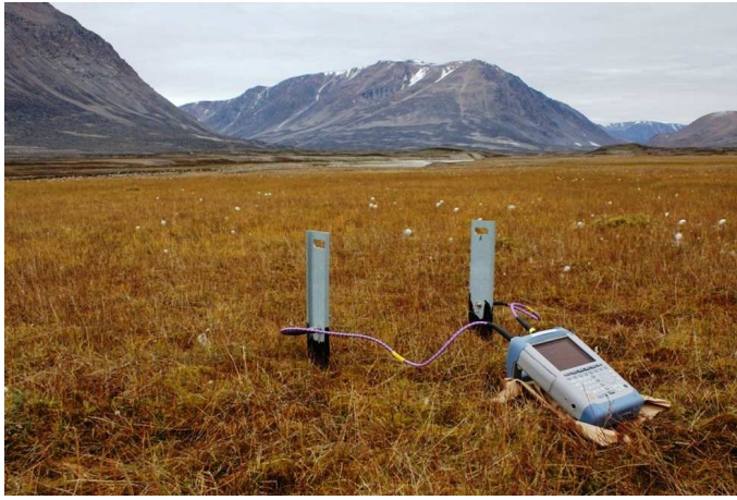
Figure 12: Photo of Zackenberg Valley in Greenland, taken on August 25th, 2009. The microwave measurement device is a Rohde&Schwarz FSH4 Handheld Network Analyzer.
