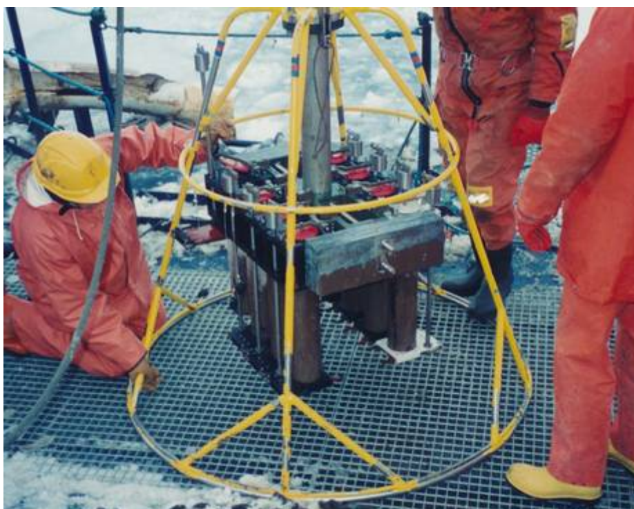
Figure 6-16 The sediment core sampler
