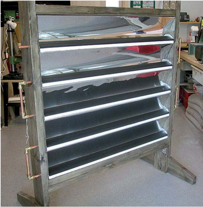
Figure 2.6 The prototype solar window with five absorbers and five reflectors. The uppermost absorber is laminated with PV cells.
