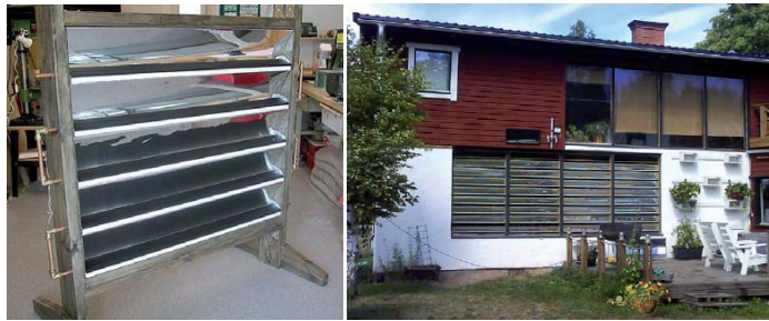
Fig 2. Left figure; the prototype solar window with five absorbers. Right figure; the solar window in Solgården with closed reflectors.
