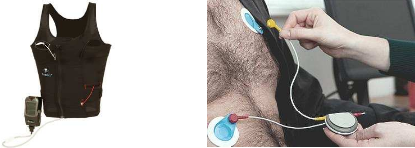
Figure 3.3 Vital signs sensor systems used in the DIAdvisor project; the VivoMetrics' LifeShirt system [VivoMetrics, 2012] (left), and the Sensium Life Pebble sensors by Toumaz [Toumaz, 2012] (right)
