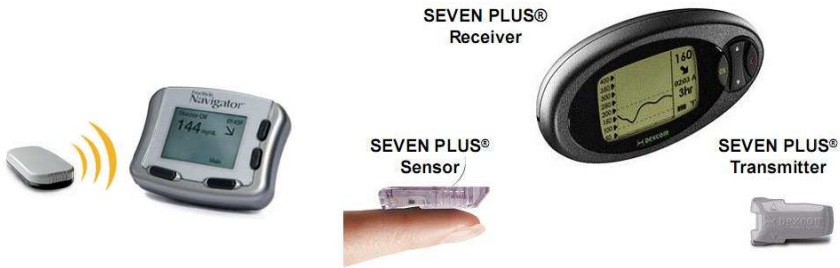
Figure 3.2 CGM systems used in the DIAdvisor project; the Abbott Freestyle CGM system, [Abbott Freestyle Navigator, 2012] (left), and the Dexcom Seven Plus CGM system [Dexcom Seven Plus, 2012] (right).
