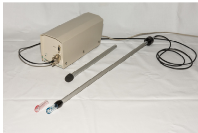
Figure 9. The acoustic rhinometry equipment shown with the nosepiece in pink or blue. Two different sizes were used depending on the size of the nose. Photo: Sigurður Júlíusson.
