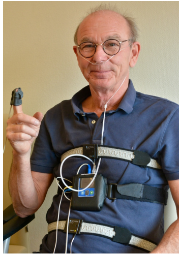
Figure 4. The placements for the different measuring signals, nose canula, thorax band, abdominal band, oximetry, and snoring by microphone. With permission of person in picture (MA).
