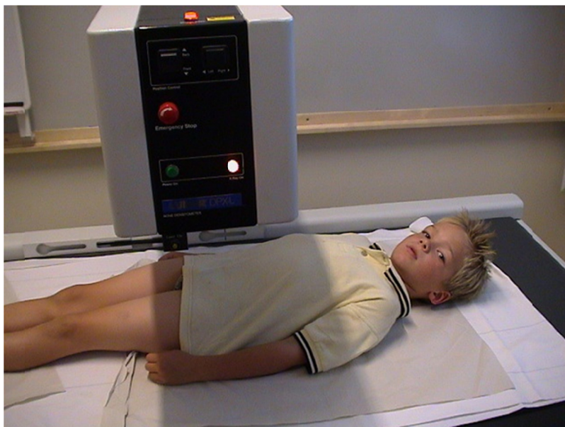
Fig. 10. The Lunar® DPX-L (DXA) apparatus Figure presented by courtesy of Christian Linden
