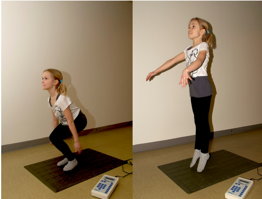
Fig. 12. VJH performed on the “Time it” Eleiko Sport® electronic mat Figure presented by courtesy of Susanna Stenevi Lundgren
