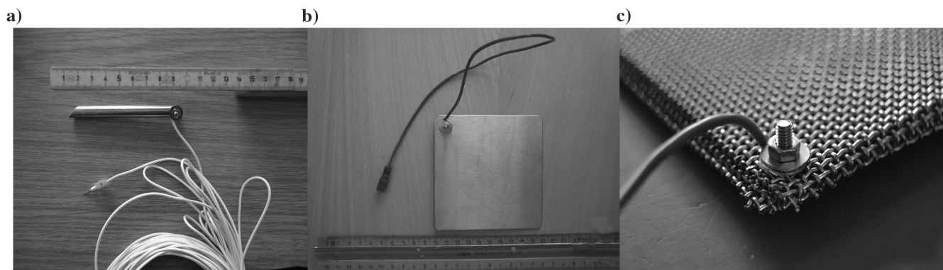
Figure 1. Electrode designs tested: (a) rod electrode with attached copper cable, (b) plate electrode, and (c) mesh electrode.
