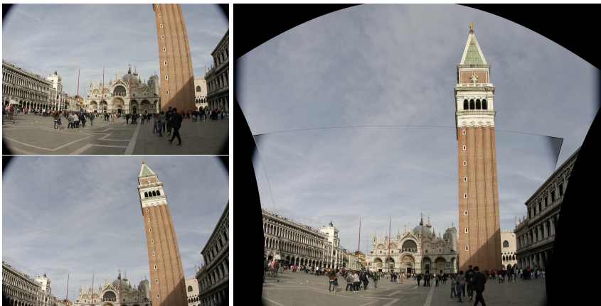
Figure 4.6: Stitching of two images with large radial distortion using on our three-point solver in a standard RANSAC framework. The resulting panorama (right) is based on the best RANSAC three-point solution without any additional non-linear refinement.
