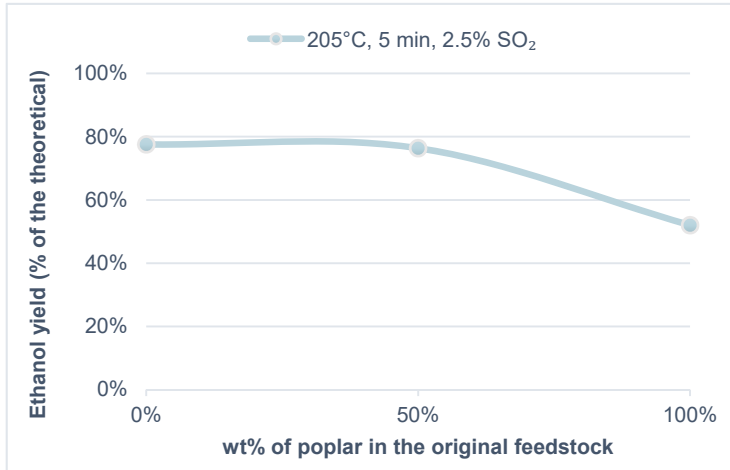
Figure 16. Ethanol yield from hydrolysate fermentation. Fermentation was performed with Ethanol Red®, an industrial hexose-fermenting S. cerevisiae strain, at 30°C, pH 5 for 96 h, at a yeast load of 5 g L -1 in shake flasks with a working volume of 50 mL, containing 0.5 g L -1 (NH 4 ) 2 HPO 4 and 1 g L -1 yeast extract. Ethanol yield is expressed as percentage of the theoretical based on all available hexose sugars (i.e., glucose, galactose and mannose) in the hydrolysates obtained from steam-pretreated spruce, poplar and a 50:50 blend.
