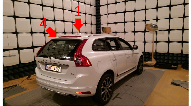
Fig. 2. The Volvo XC60 and the positions of two receiving antennas used in the measurement.
