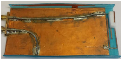
Fig. 7. 130mm x 66mm x 8mm fabricated polycarbonate chassis with 20mm rotationally symmetric capacitive loading offset.
