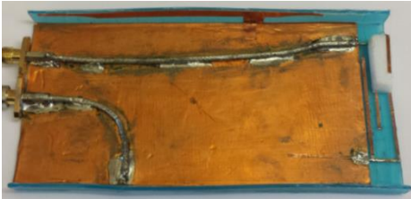
Fig. 7. 130mm x 66mm x 8mm fabricated polycarbonate chassis with 20mm rotationally symmetric capacitive loading offset.
