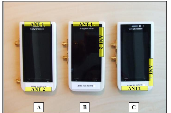
Fig. 3. Location of the antennas for each of the three multi-antenna configurations in the terminal prototypes.
