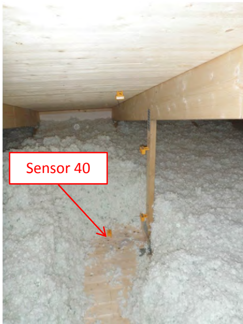
Figure 9.40.5. Location of the studied position. The cellulose fiber insulation was temporary removed.
