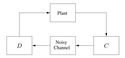
In this problem, the objective is to design an observer/coder C and decoder/controller D that stabilize the plant and minimizes the effect caused by a plant disturbance (not shown).
