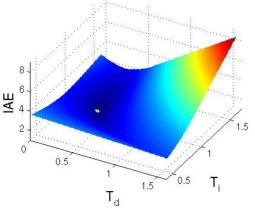
Surface plot from the PID design tool
