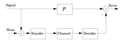
The objective is to design the coder and the decoder so that the estimation error is minimized. This can be interpreted as a real-time coding problem (if P is replaced by a time delay) with input noise. Another interpretation is that this concerns the design of a disturbance feedforward compensator, where the sensor and the actuator are geographically separated.
