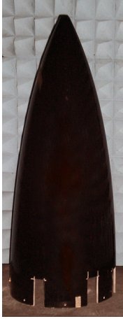
Figure 13: The radome diagnosed in Papers I-IV. The missing pieces at the bottom have been used for material characterization.
