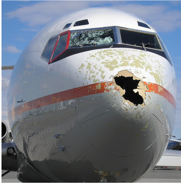
Figure 6: The nose cone of a cargo Boeing airplane, after flying through a severe hail storm. Photo courtesy of Dave Subelack.
