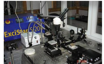
Figure 5.3. The FBG fabrication system at Zhejiang University.
