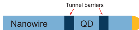
Figure 1.2: A quantum dot in a nanowire defined by two thin segments (dark blue) of a different semiconductor compound (heterostructure) or crystal phase (homostructure).
