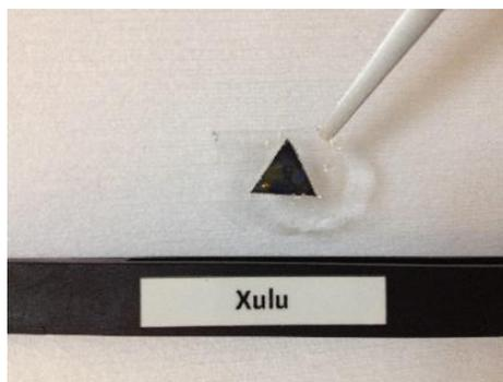
**Figure 15.** A peeled-off FC film with nanowires embedded in the triangular area.
