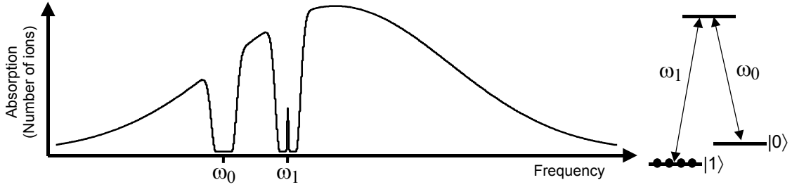
Figure 3.4. A group of ions is prepared in a specific ground state sublevel, |1\rangle , and the surrounding spectral interval is emptied of other ions, using spectral hole-burning. Another pit in the inhomogeneous absorption profile is created in the around the frequency where the ions will absorb if they are in ground state sublevel |0\rangle . The selected ions can now be manipulated using light with frequencies \omega_0 and \omega_1 .
