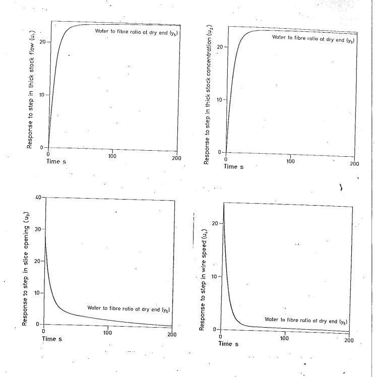
Fig Q.3 Normalized stepresponses in moisture content for the linearized paper machine model. The input amplitudes are chosen equal to the steady state values and the outputs are normalized with respect to their steady state operating levels.
