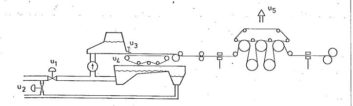
Fig. 2.1 - Simplified diagram of a paper machine.
