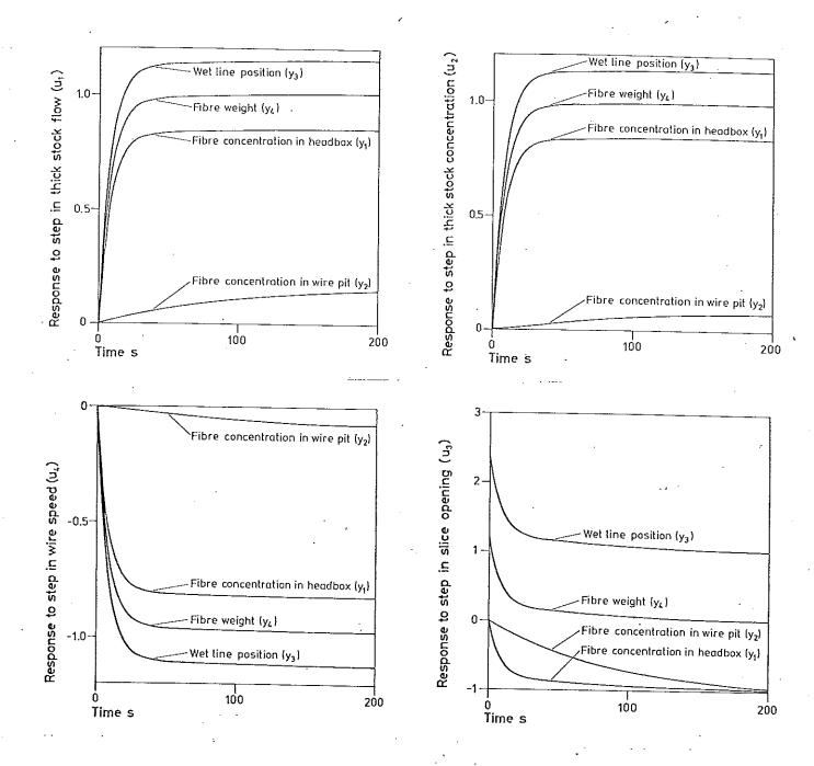
Fig 2.2 Normalized stepresponses for the linearized papermachine model. The input amplitudes are chosen equal to the steady state values and the outputs are also normalized with respect to their steady state values.
