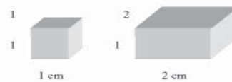
Figure 1. Effect of bone size on measured bone mineral parameters in a section of bone 1 cm long. Both bone samples have identical volumetric densities (true bone mineral density); however, the bone mineral density (BMD) of the larger sample is twice that of the smaller sample. Adapted from Carter et. al. 1992.
