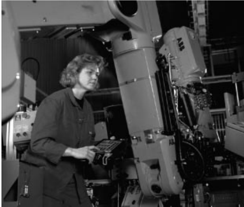
Figure 2.3 Robot operator/programmer at Volvo, Sweden, doing on-line changes of robot motions for gear-box assembly, using ABB Irb-3000 robot systems. (With permission from ABB and Volvo.)
