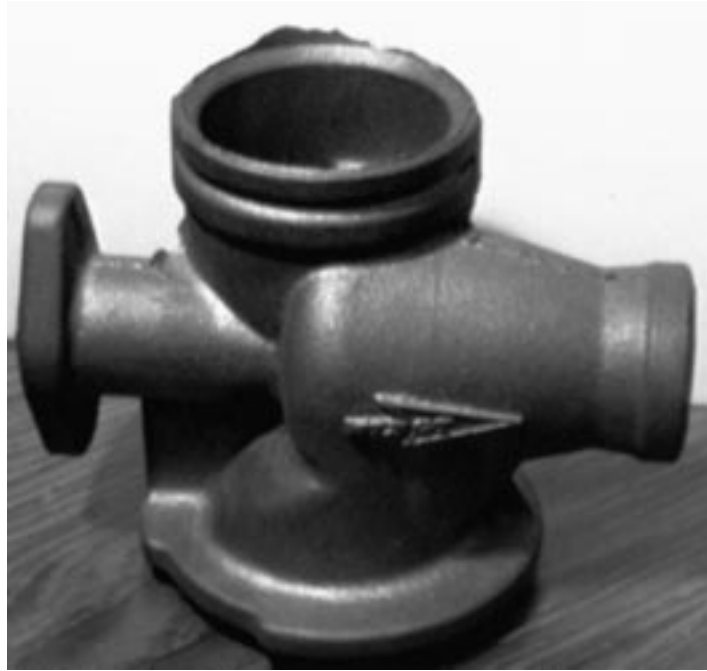
Figure 2.4 Valve housing from Flygt, Sweden, with burrs remaining from the sand casting. The height of the piece is approximately 170 mm.
