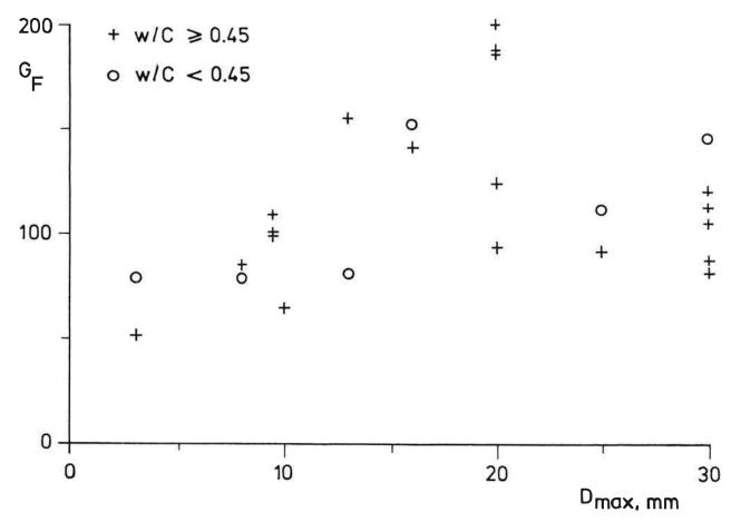
Fig. 2 Variation of  $G_F$  with maximum aggregate size and water/cement-ratio for standard beams according to the draft recommendations.
