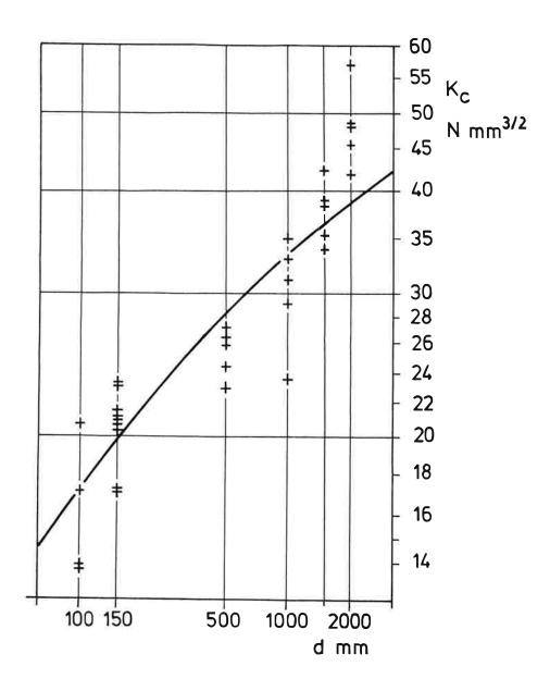
Fig. 1  $K_c$  according to the Bologna tests as a function of the beam depth. The curve shows a theoretical relation for E = 24.6 GPa,  $G_F$  = 160 N/m,  $f_t$  = 2.1 MPa according to /3/.
