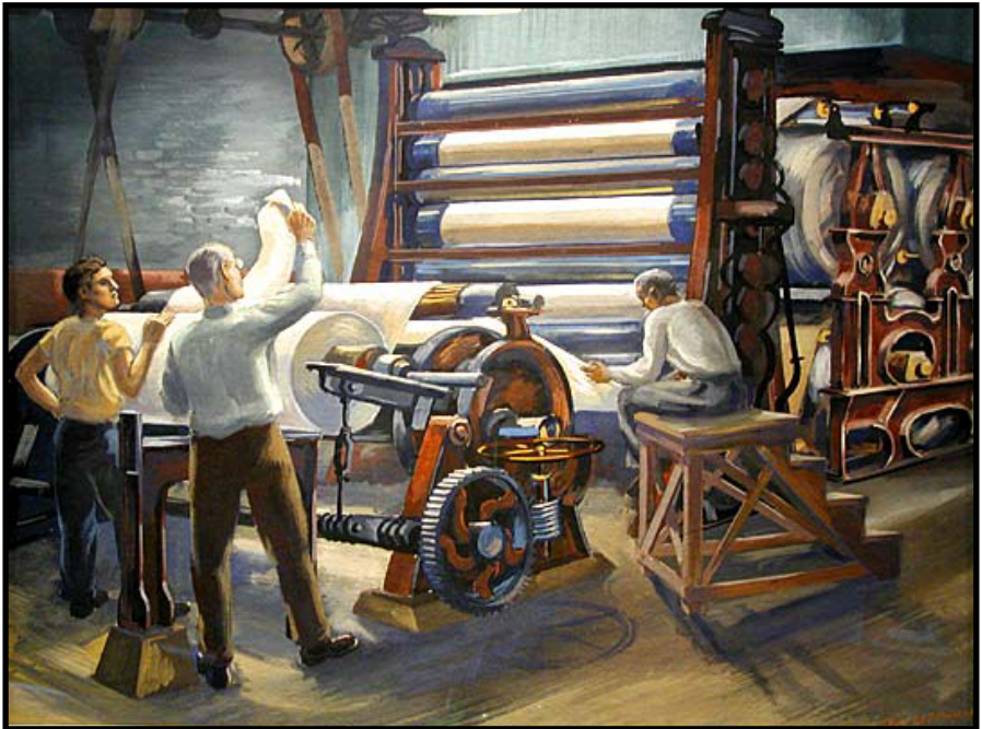
Papermaking in the early 1900s, painted by Thomas M. Dietrich. It shows the dry end of the paper machine at the Fox River Paper mill in Appleton, Wisconsin. The man is checking the feel and transparency of the sheet for its thickness and formation. The paper has moved from right to left in this painting, passing through the dryers, calender stack, and reel. By courtesy of Fox Valley Corporation.
