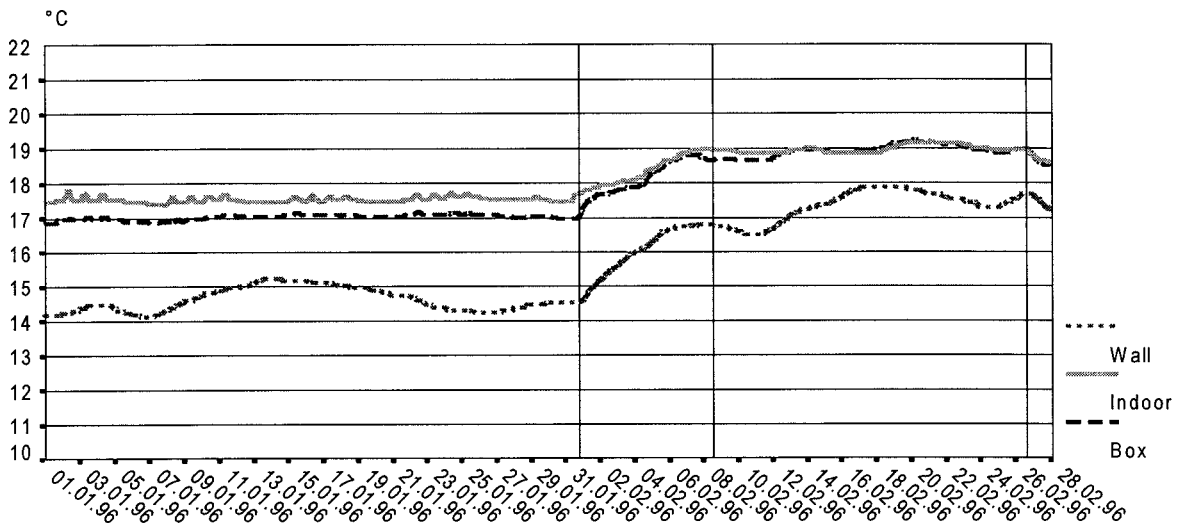
Figure 32 The course of the temperature in the masonry wall, the indoor temperature and inside an archive box.
