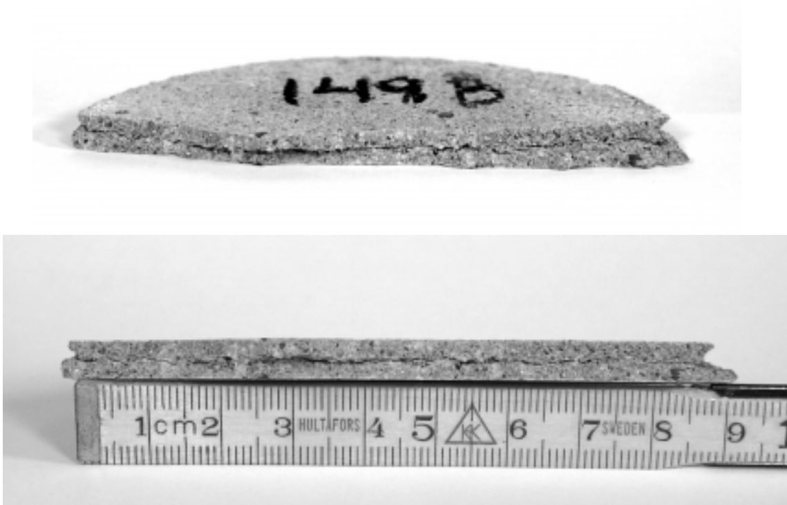
Figure 7.1.31: Crack in the center of w/c ratio 0.65 specimen stored in 3% NaCl solution for 19 days prior to test at -10^{\circ}\text{C} , bath salt concentration 14.4%. (Two views)
