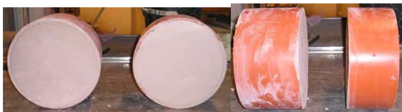
Figure 6.1 Samples to the rendering-experiment. Each tube has thermal insulation inside the tube and mortar applied on each side
