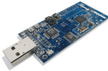
Figure 1.15 The Telos B mote is a low power wireless module, equipped with an 8 MHz Texas Instruments MSP430 microcontroller with 10 kByte RAM and 48 kByte Flash memory.
