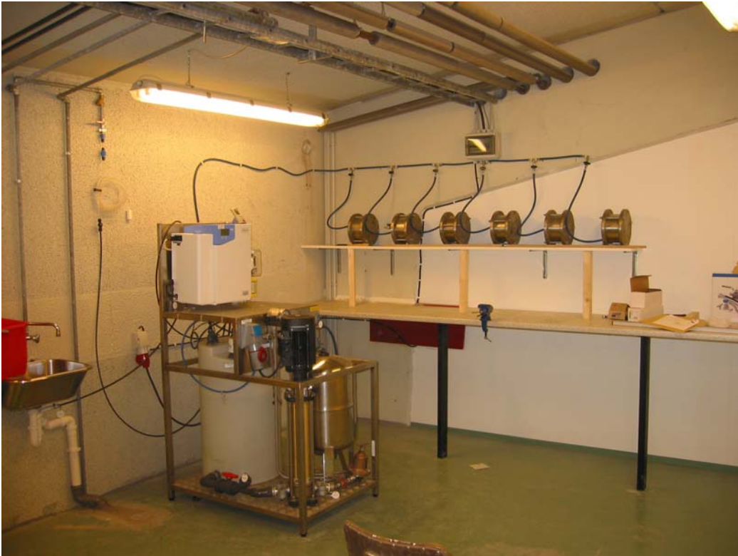
Fig. 2 Photo of the test rig built in Sweden for delivery to Iceland, comprising water purifying part, pump, pressurized water storage tank and pressure reducing units.
