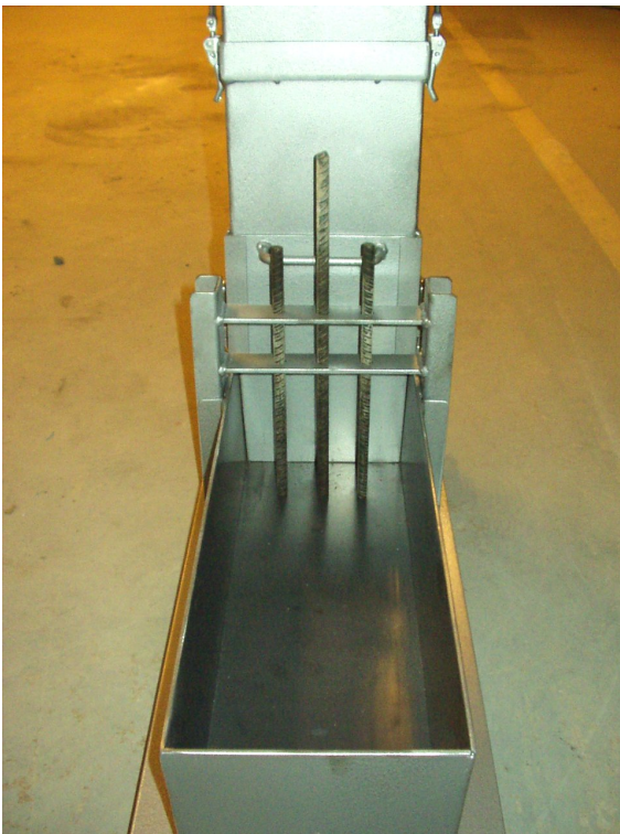
Fig. 3.4 – Bottom of L-box filled with water before a sliding gate was opened at the end of the box in order to cast concrete in the vertical shaft submerged in the box and to cure it there.
