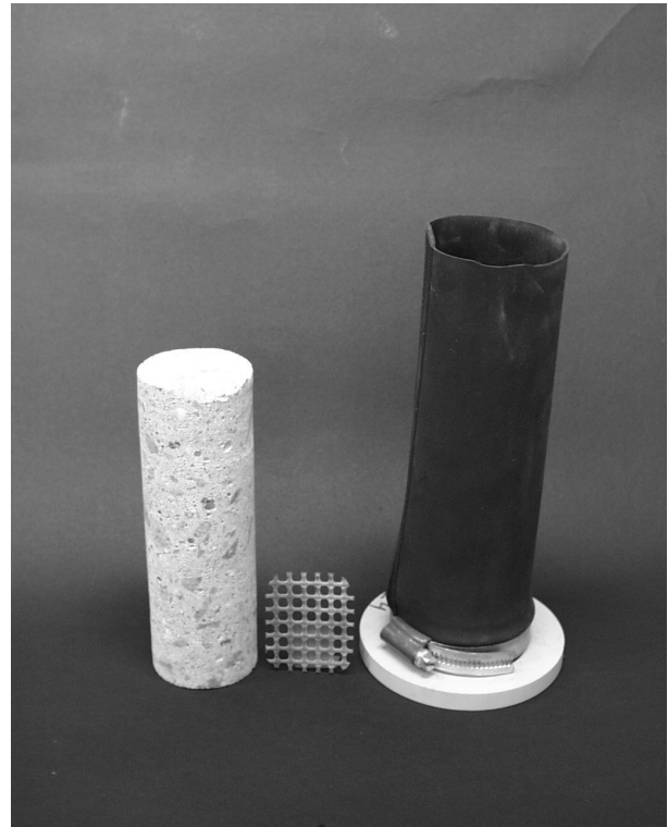
Fig. 3.7 - Specimen in rubber container, immersed in distilled water (internal frost resistance tests).
