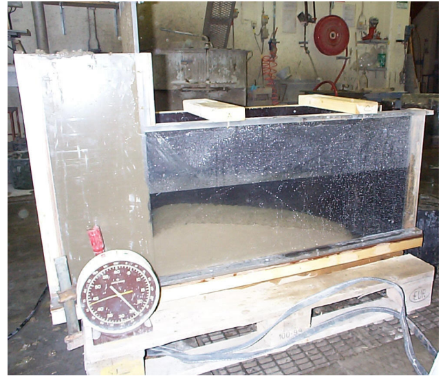
Fig 2.70 - Modified L-box apparatus with underwater concrete without anti-washout additive [85].
