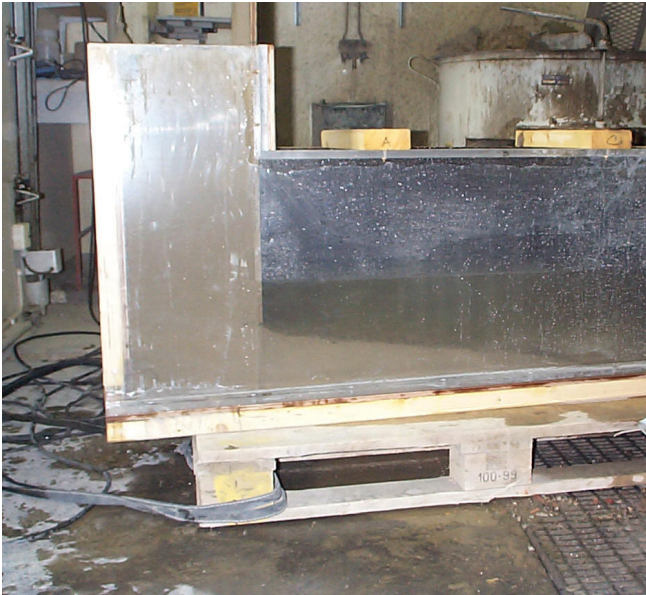
Figs. 2.69 - Modified L-box apparatus with normal concrete K40 [85].
