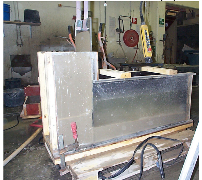
Fig. 2.72 - Modified L-box with SCC (slump flow 570 mm 570 mm only) [85].
