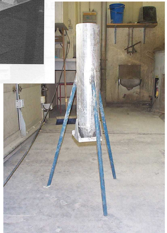
Fig. 2.68 - Orimet test apparatus - a flow ability test also used for SCC [85,92].
