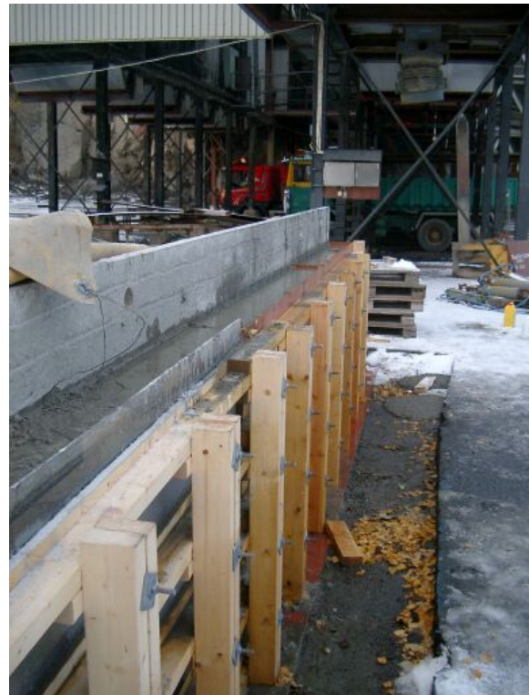
Fig. 3.6 – Field test at BTC with one side of mould consisting of a prefabricated concrete element and the other of wood or transparent glass fibre. Photo: Iad Saleh.
