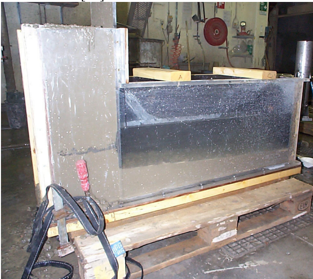
Fig. 2.71 - Modified L-box with underwater concrete with anti-washout additive [85].
