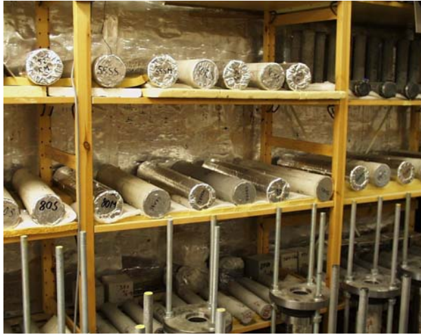
Figure 3.11 - Specimen for studies of long-term shrinkage.
