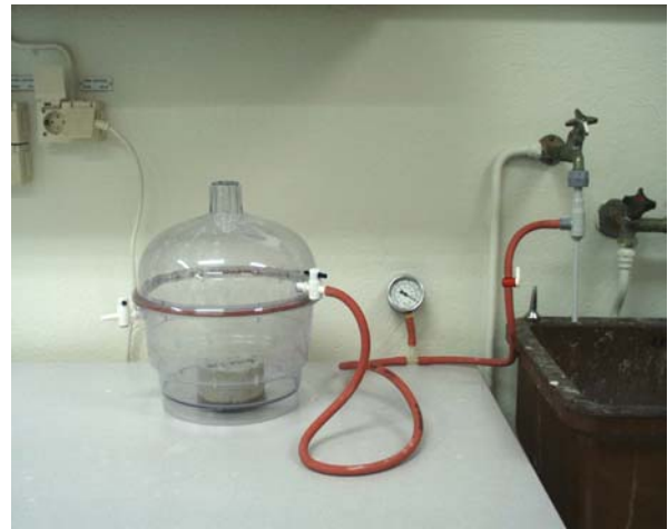
Figure 3.1 - When the specimens were surface-dry, they were placed in a vacuum container to a pressure in the range of 1-5 kPa within a few minutes [4].
