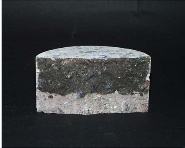
Figure 3.7 - Specimen for test of the chloride migration coefficient, D [4].
