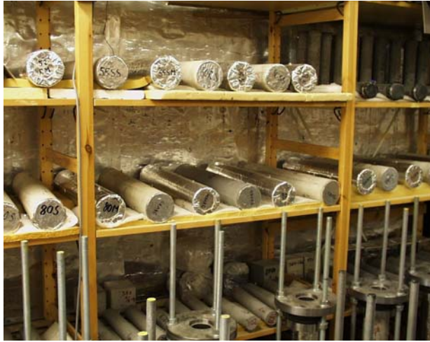
Figure 3.11 - Specimen for studies of long-term shrinkage.
