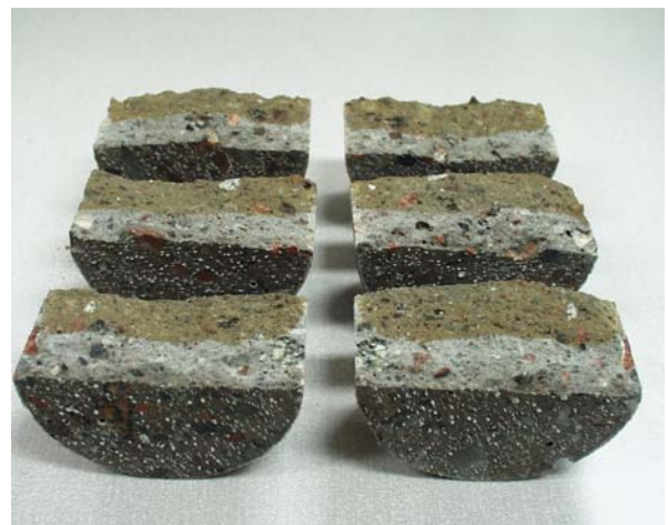
Figure 3.6 - Test specimen after preparation for chloride penetration depth measurement [4].
