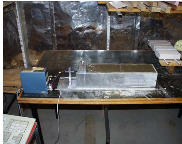
Figure 3.10 - Equipment for shrinkage measurement of up to 1 day's age.
