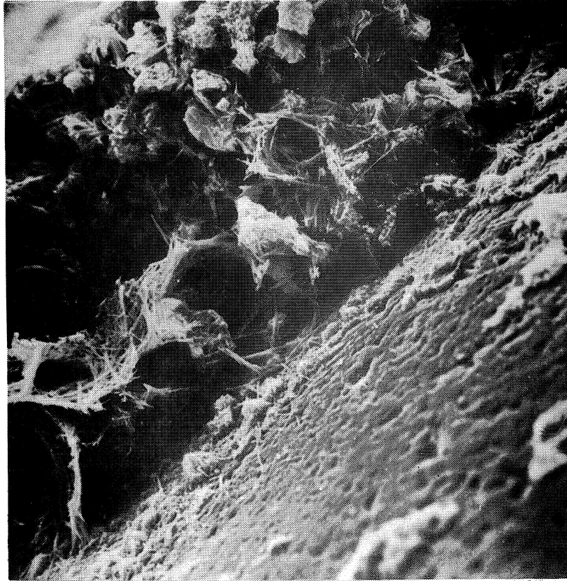
Fig 64: Scanning electrone microscope picture of cement mortar. 1:4. W_o/c = 0,54 . Porous interface paste - grain of aggregate. The grain to the right. Photo: Inst of Zoology. Univ of Lund.
