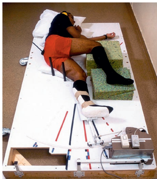
The tests of knee proprioception were done with the test person in a lateral decubitus position on a specially-designed platform. This test person is not a participant in the study.
