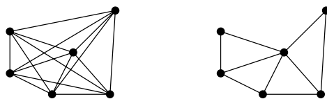
Figure 1.2: Example of a t -spanner of the complete Euclidean graph with t = 1.18 .
