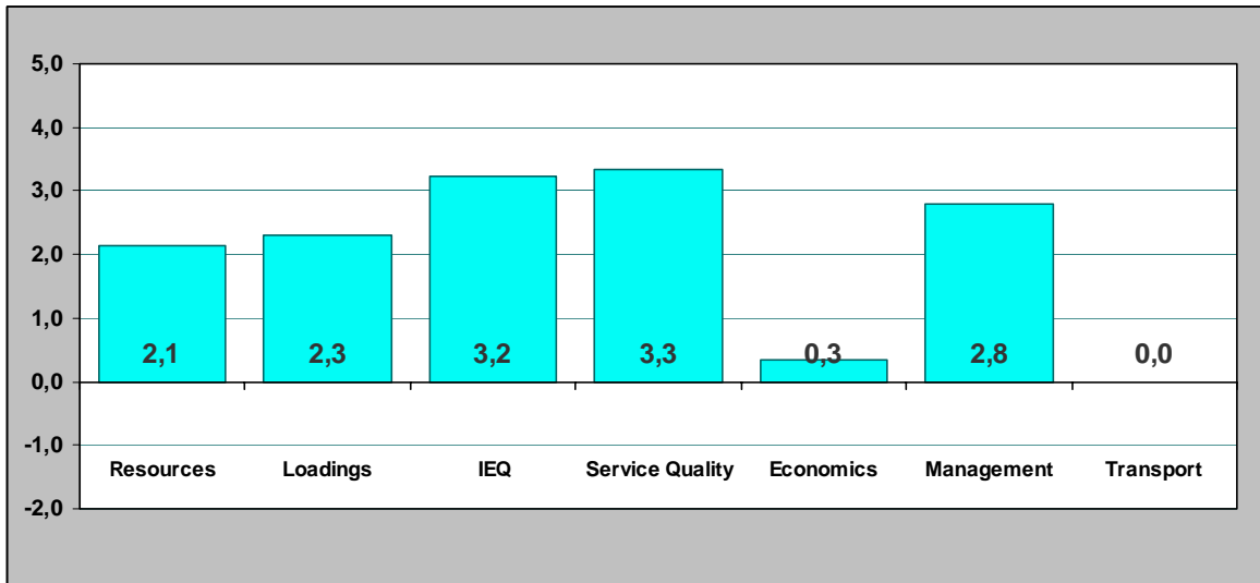
Figure 2.7 GBTool – concluding result diagram. 'Loadings' indicate global environmental aspects such as green house effect or ozone depletion. 'IEQ' = Indoor environmental quality, 'Service Quality' refers to aspects such as access to daylight and flexibility. 0 indicates minimum quality for new buildings according to norms and 5 the best available technology. (iiSBE, 2003).
