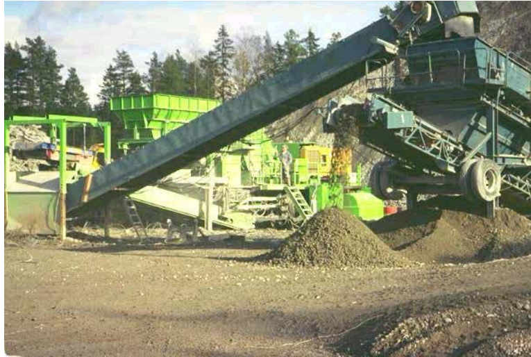
Figure 4.8 Recycling of hardened concrete. After coarse crushing the reinforcement is separated magnetically (rack to the left) and then the material is further crushed (right) to the desired particle size. Photo by the author.
