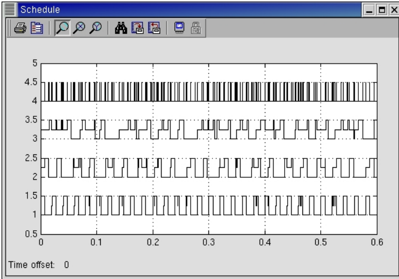
Figure 7.5 Example of an execution trace generated by a computer block during a simulation. The example involves three periodic tasks. The upper graph shows the execution of the kernel simulating context switches.
