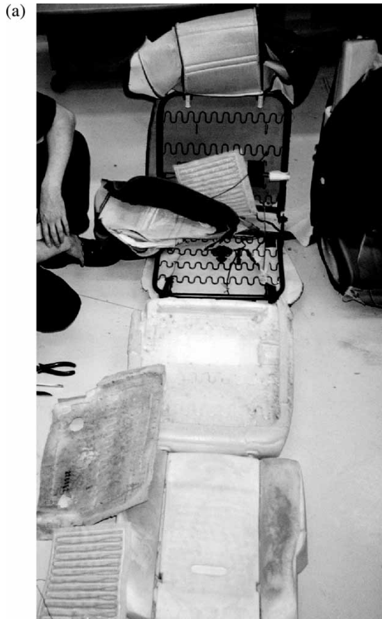
Figure 2. Car seats: (a) simple old seat (1996); seat foam not integrated in the frame; zipper to remove the outer material without cutting; no electric devices; (b) complex newer seat (produced today); to the left : back panel embedded in the seat frame, to the right : numerous electric components.
