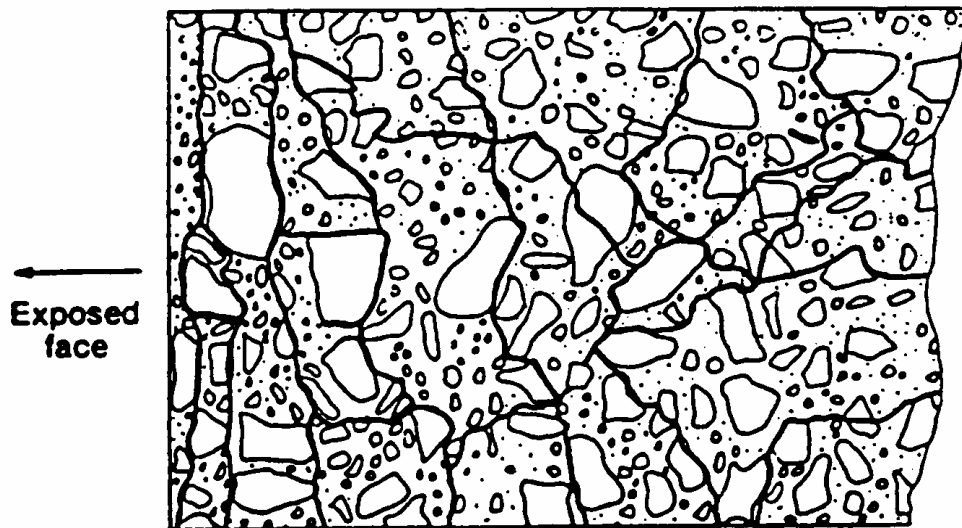
Figure 2: Typical internal crack pattern induced by frost action.
