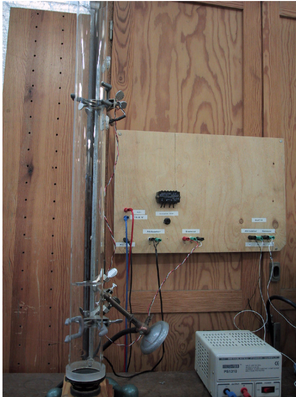
Figure 5.15 Photo of Rijke Tube rig
