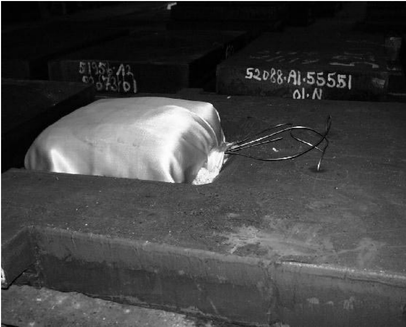
Figure 9.1 The data collection device mounted on a test slab. The wires going into the slab are the steel coated thermocouples. The water box is covered heat protective material to minimize the exposure to heat radiation.
