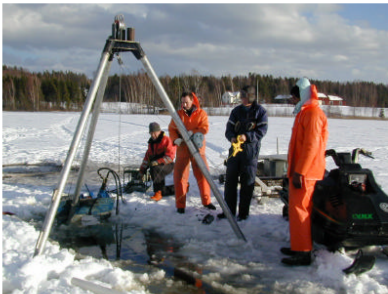
Joint Swedish and Finnish fieldwork on the ice covered Lake Kälksjön, Värmland, west central Sweden, March 2002. Retrieving a sediment piston-core for palaeomagnetic measurements.
