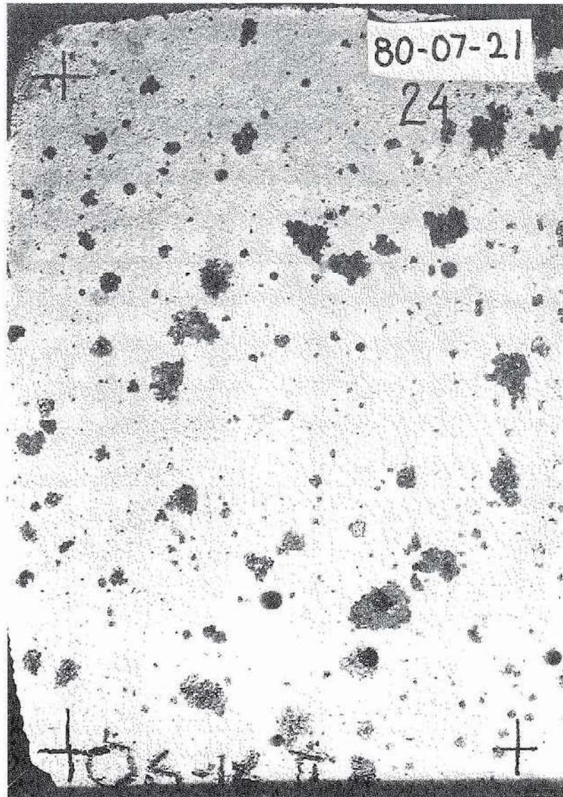
FIG 3.2.3 Surface of specimen No 6:24, sealed cured for one week and then stored in 100 % RH at +20°C, showing no pop-outs whatsoever but many gel extrusions.
