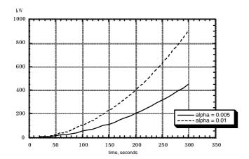
Figure 6. Energy release rates using the mean values of the fire growth rates.
