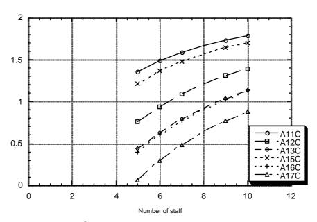
Figure B29. Reliability index  $\beta$  for different patient categories in corridor scenario with open door and detector failure.
