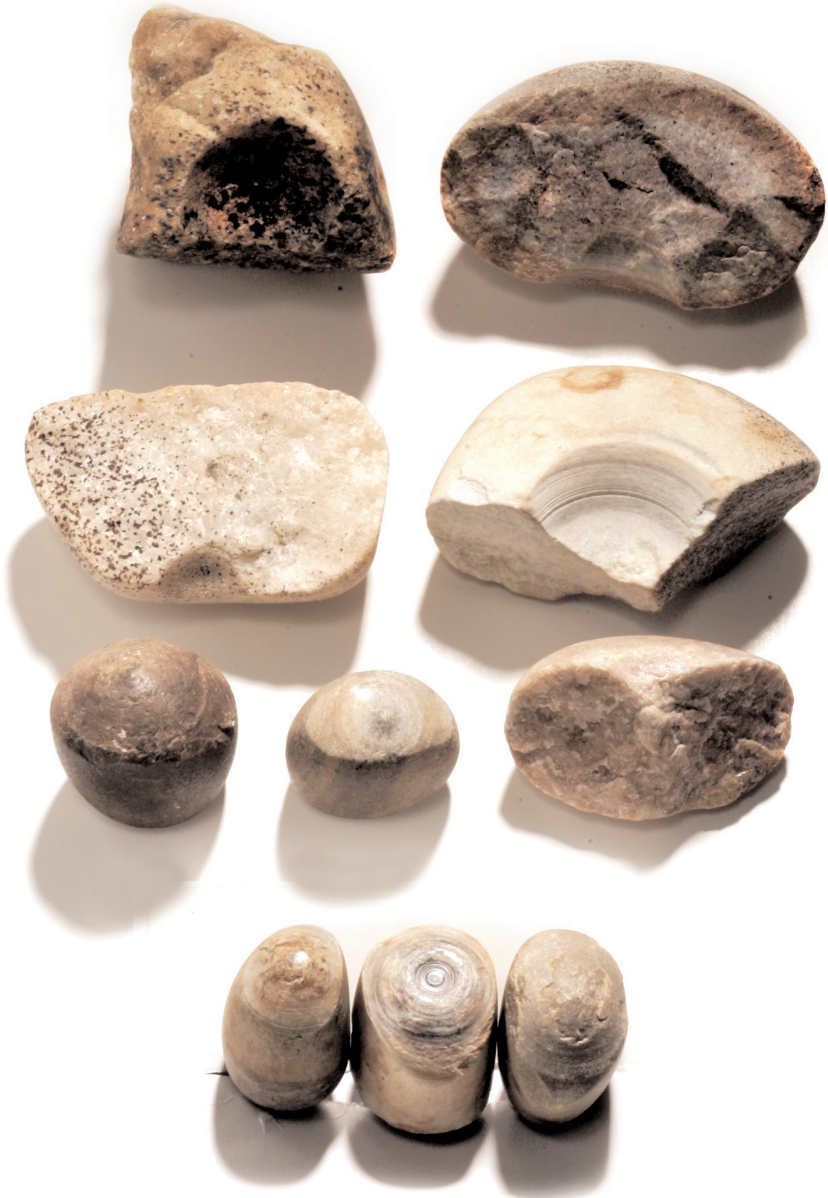
Fig. 3. Stone artefacts used during earlier times in the rotating machinery of the mill. All were collected under the water flowing only a few meters from the mill. First and second upper rows: four parts of circular stones belonging to the driving machinery. Third row: two small ovoid stones (highly polished) and a piece of a circular stone. Fourth row: three other small egg shaped stones which are also highly polished, some of them on both sides.
